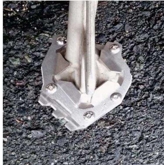
Add thread locker to the tip area of each screw. Arrange side stand foot in place. Start the two screws closest to the bike (at the tips of the upper plate) by hand. Then place and start the rest of the screws but do not fully tighten yet.
